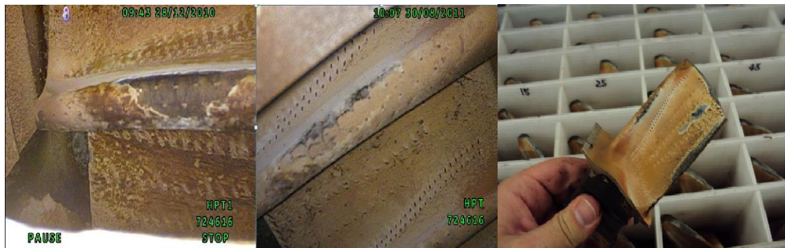
Figure 8 - Deterioration progress in a first stage blade of the HPT
