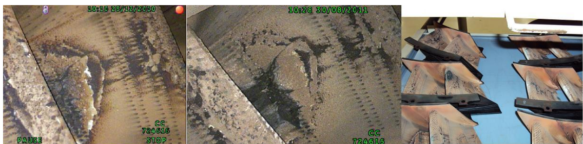
Figure 9 - Deterioration progress in first stage NGV of the HPT
