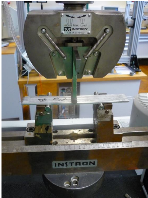
Figure 3.9 – Bending runs set-up and composite test samples dimensions.
