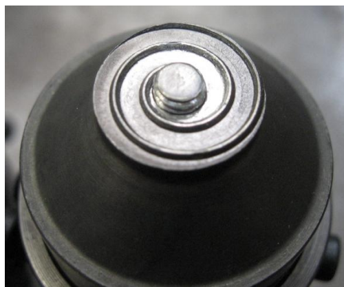
Figure 3.4 – FSW used tool, 18 mm diameter plain shoulder with one two-lap ridge, and a 5 mm diameter threaded cylindrical pin.
