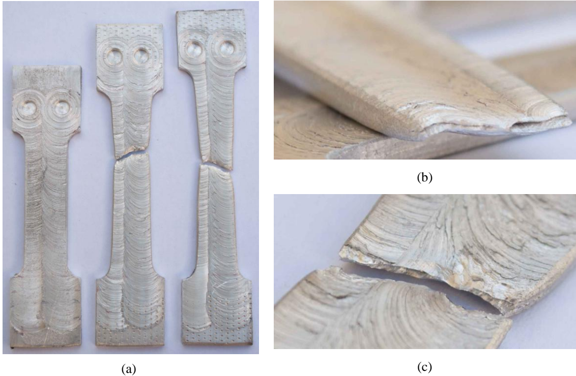
Figure 4.14 – Aluminium lap joint tensile test samples; (a) overlapping FSW by the AS, from left to right, untested sample, 1800 KN axial force FSW tested sample, 2000 KN axial force FSW tested sample; (b) detail of 2000 KN sample, (c) detail of 1800 KN sample.
