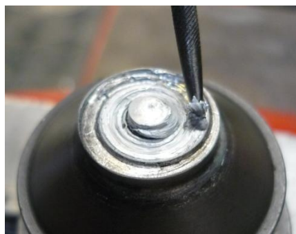
Figure 4.26 – Tool threads cleaning after a set of trials, AA 1100 remnant material is being removed with a scriber tool.
