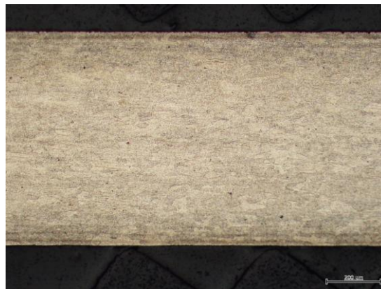
Figure 4.1 – As-received AA 1100 cold hardened and partially annealed, section parallel to rolling direction
