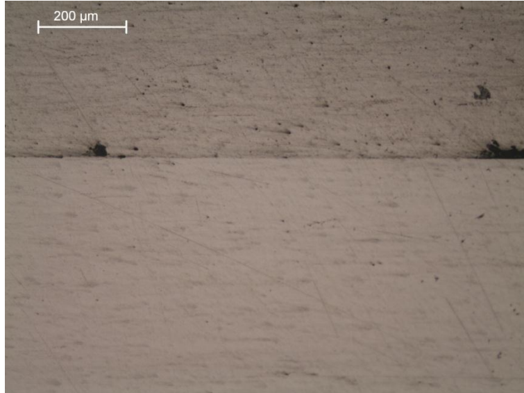
Figure 4.10 – Interface defects detail from coating D17
