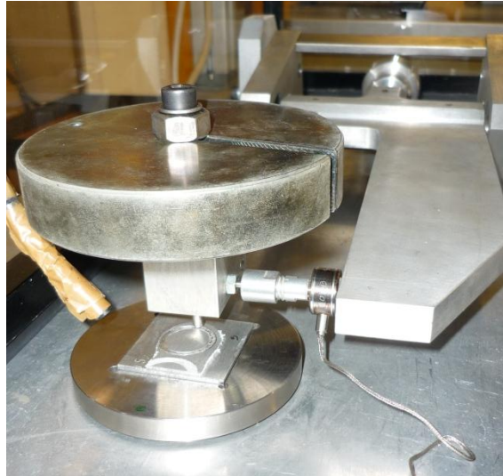
Figure 3.5 – Detail from the wear machine used
