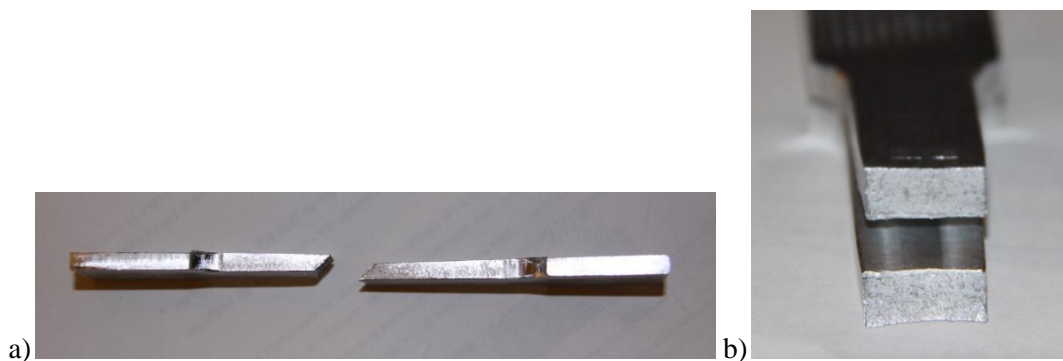
Figure 4.31 – Tensile sample: a) tested specimen, b) fracture section
