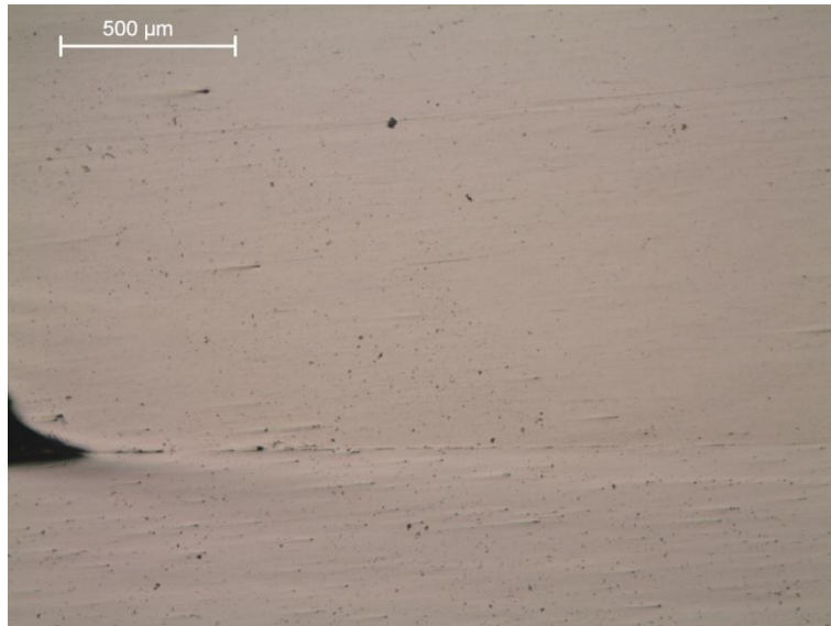
Figure 4.7 – Detail of the edge coating D14.
