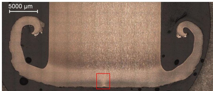
Figure 4.18 – Macrograph of CD5 sample
