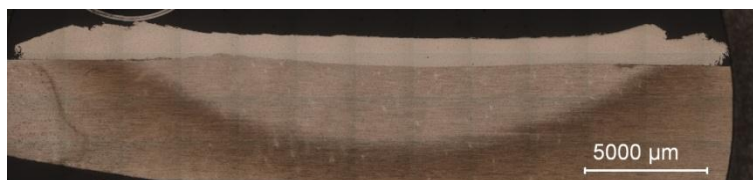
Figure 4.21 – Substrate HAZ of coating D24
