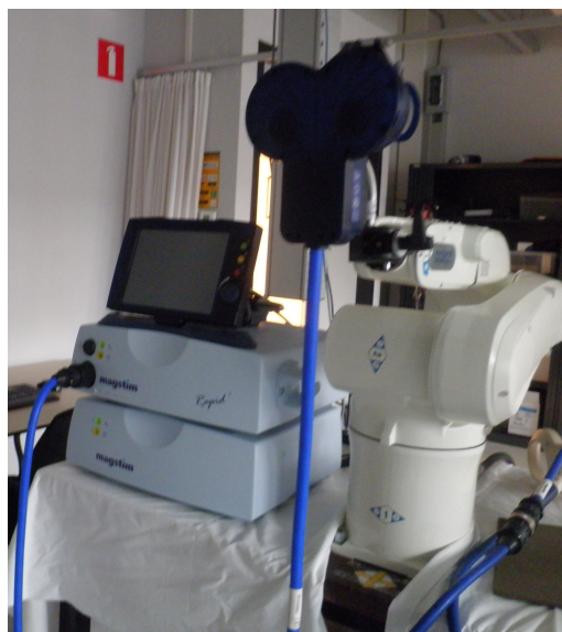
Figure 3.3: The magnetic stimulator with the touch screen interface. The robot-navigated system is used for accurate positioning of the figure-of-eight coil.
