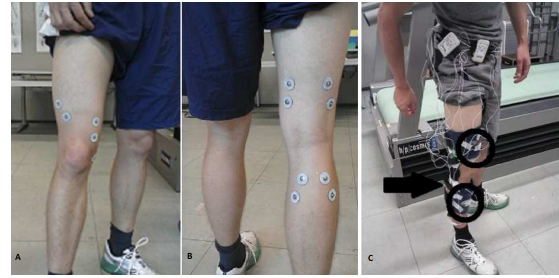
Figure 1: (A, B) Placement of electromyography surface electrodes (C) Complete experimental setup: two Bioplux research devices, two ACC (circles), six EMG and one goniometry sensors (arrow) placed on a regular Ortema right knee orthosis
