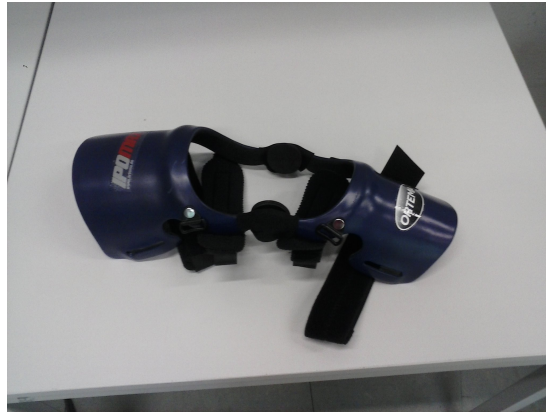
Figure 3.1: Standard right knee Ortema ipomax passive orthosis
