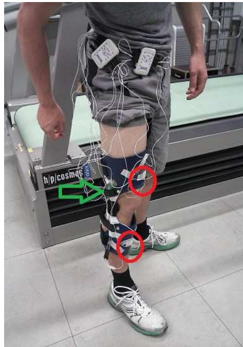
Figure 3.2: Complete experimental setup: two Bioplux research devices, two ACC (red circles), six EMG and one GON sensors (green arrow) placed on a regular Ortema right knee orthosis
