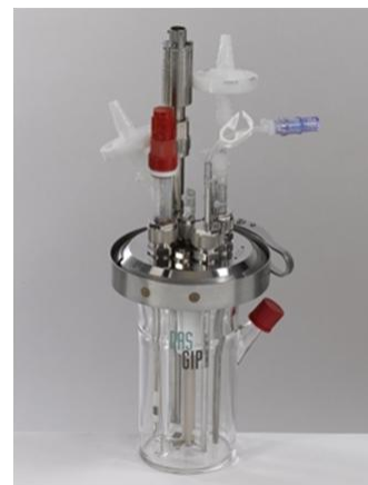
Figure I.7: Suspension culture systems: rotary culture system (a) and stirred culture system (b). Adapted from http://www.thco.com.tw and from http://www.dasgip.com/catalog/ .
