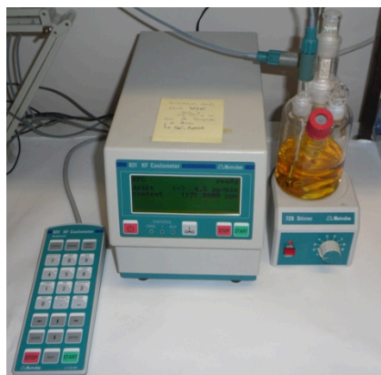
Figure 2.1 - Metrohm 831 Karl Fisher coulometer used.
