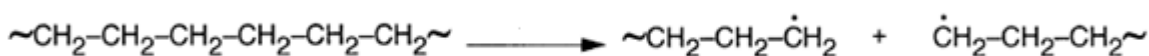
Figure 1.5 - Illustration of the initiation step according to a free radical chain mechanism for PE thermal degradation [adapted from (Bockhorn, Hornung et al. 1999)].
