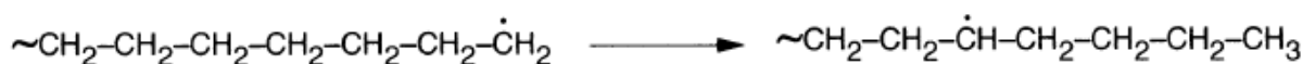
Figure 1.6 – Possible paths that allows the \beta -scission of the more radicals, resulting a primary radical and an olefin [adapted from (Bockhorn, Hornung et al. 1999)].
