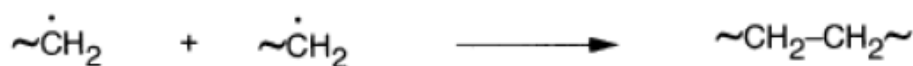
Figure 1.9 – Termination step according to a free radical chain mechanism (adapted from (Bockhorn, Hornung et al. 1999)).
