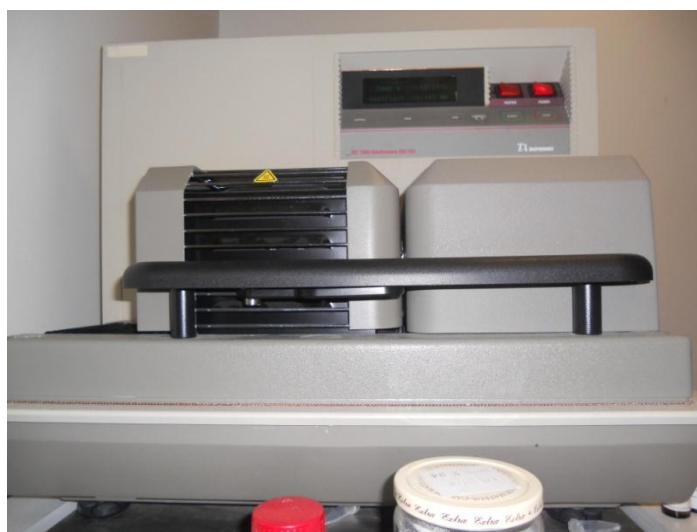
Figure 2.5 – TG/DSC instrument (TA Instruments ® SDT 2960).
