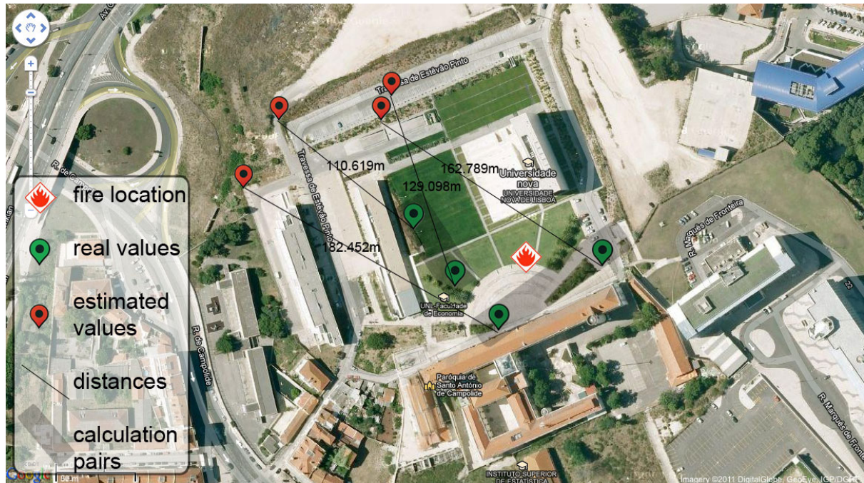
Figure 16 - Visualization of estimated Origin Points (GPS Readings) in relation to real values
