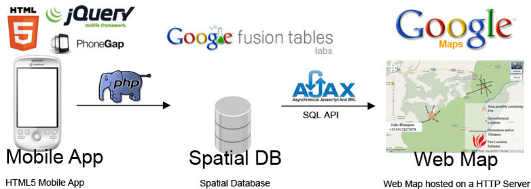
Figure 7 - Technological Architecture of the FireSpotter System
