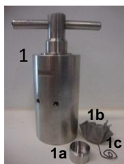
Figure 5.3. High-pressure cell and components used during impregnation tests (1- High-pressure cell; 1a- basket; 1b- metallic net; 1c- wire support).
