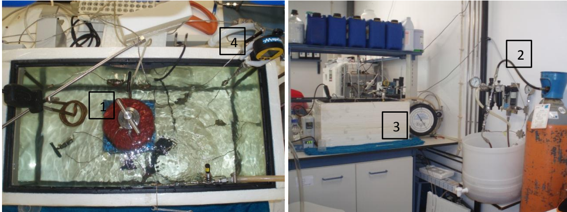
Figure 5.1. Image of installation where the tests were performed (1- High-pressure cell; 2- CO 2 pump high pressure liquid; 3- Thermostated water bath, 4- Pressure manometer).
