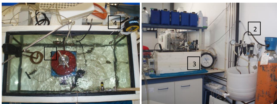
Figure 4.1. Image of installation where the tests were performed (1- High-pressure cell; 2- CO 2 pump high pressure liquid; 3-Thermostatized water bath, 4- Pressure manometer).
