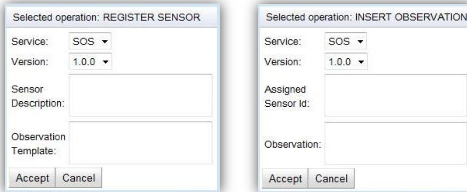
Figure 13: Overlapping windows for Transactional Profile operations. The blank fields have to be used for inserting XML code.
