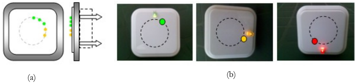
Figure 5-7 Wall illuminated light switcher prototype (a) drawing and (b) LED functionality experimentation (In Hipolito 2008)
