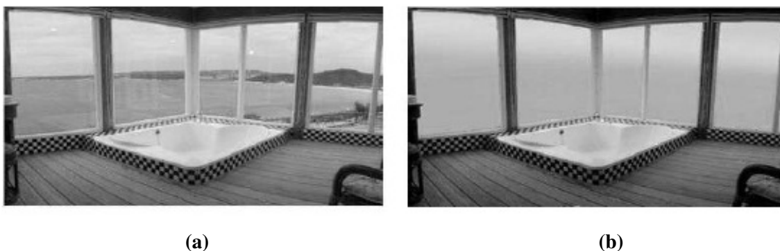
Figure 1.18 – Example of application of PDLC in switchable windows in ON (a) and OFF (b) state.
