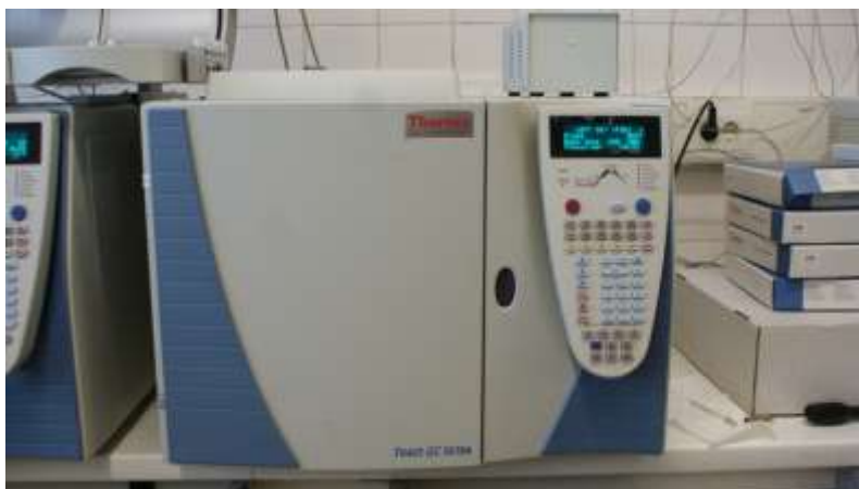
Figure 2.2.5: Gas Chromatograph on-column THERMO SCIENTIFIC TRACE GC ULTRA
