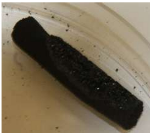
Figure 3.1.5: SCG after experiment at 603.15 K, 10 MPa, 1ml/min methanol
