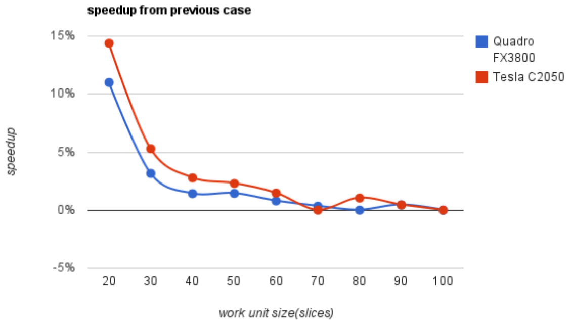
Figure 3.8: Processing speedup from previous case of a 512^3 samples dataset using different work unit sizes.
