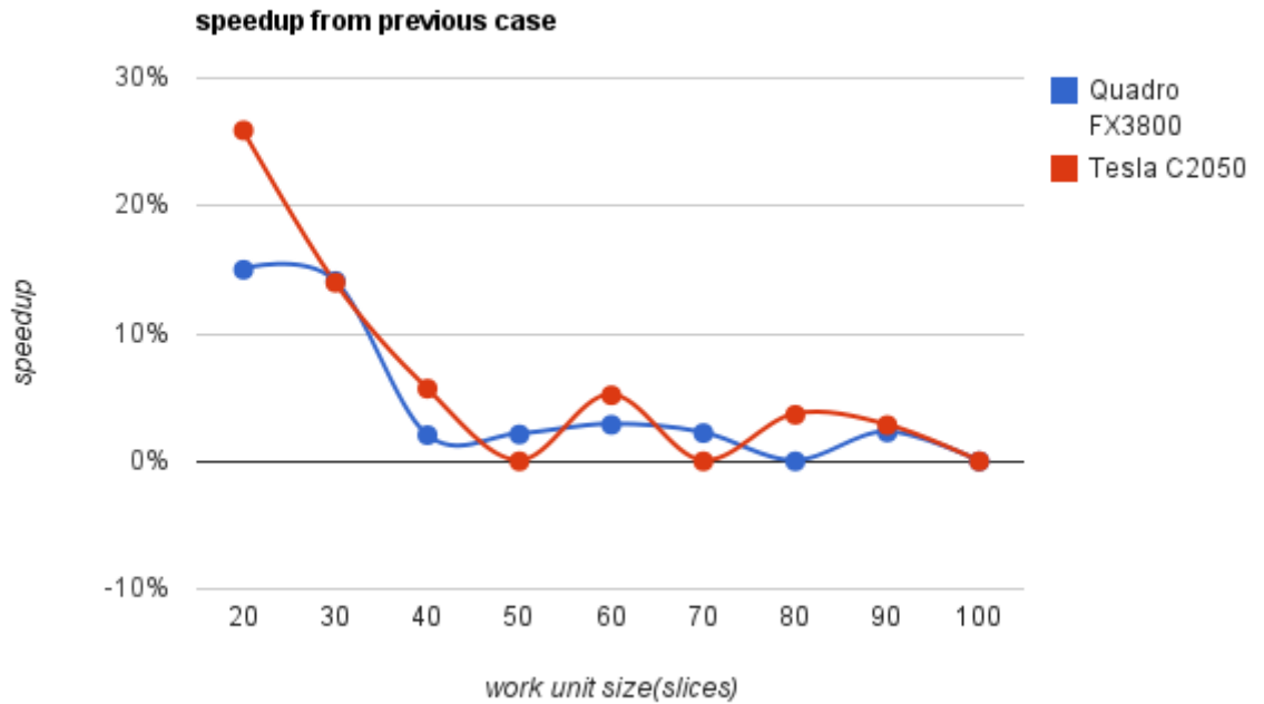
Figure 3.5: Processing speedup from previous case of a 256^3 samples dataset using different work unit sizes.
