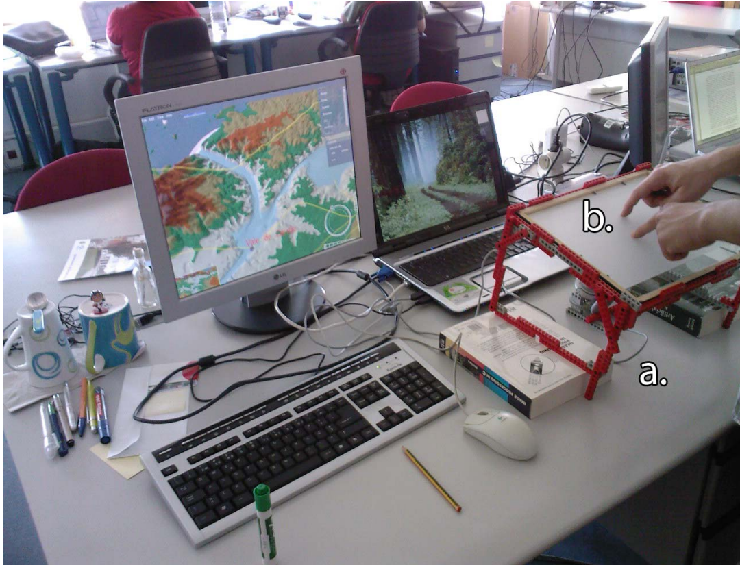
Fig. 5.4 – Multi-touch input device. a) Camera, b) Touchable area.
