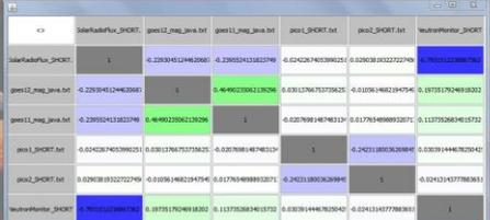
Fig. 2 - Correlation matrix view. This displays the pairwise correlation between all the loaded time series. It provides a colour representation of positive (green scale) and negative (blue scale) correlations, with stronger colours representing higher correlations.
