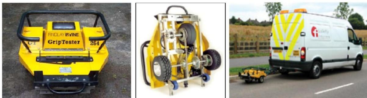
Figura 4.13 - Equipamento *Grip Tester* (Alves, 2007; Findlay-Irvine, 2007)
