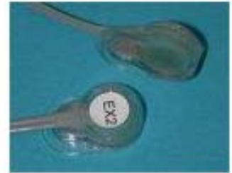
Figure 6.2 - Flat-type active-electrodes. Extracted from http://www.biosemi.com/active_electrode.htm
