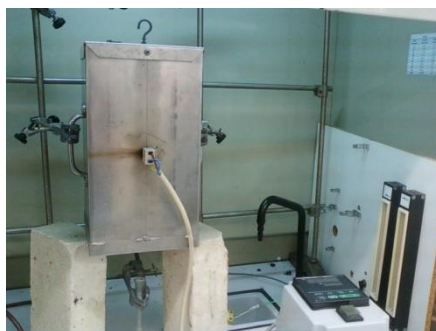
Figure 3.4. Tubular oven used in the procedure to modify the AC (FCT/UNL).
