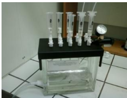
Figure 3.5. Solid phase extraction apparatus used in the experiments (Sanitary Engineering Laboratory (LABES) of the Urban Water Division (NES) of LNEC's Hydraulics and Environment Department (DHA)).
