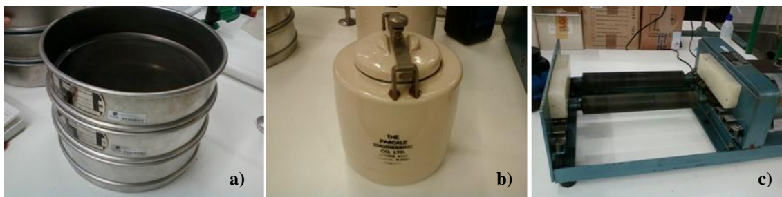
Figure 3.2. Retsh Sieves (ASTM E-11) (a); Ceramic Ball Mill (The Pascall Engineering Co, Ltd) (b); and Ceramic Ball Mill holder (c) (Chemistry Department of the Faculty of Sciences and Technology – New University of Lisbon).
