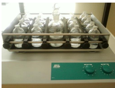
Figure 3.6. Apparatus used in the kinetic and isotherm batch experiments ( Edmund-Bühler orbital shaker).
