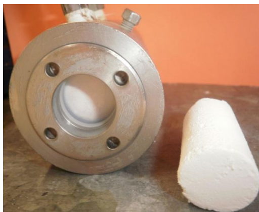
Figure 2.3 - High-pressure reactor used in the polymerizations and typical P(MAA-EGDMA) with molar ratios of 1:32:20.
