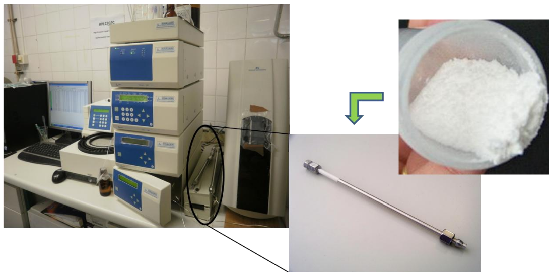
Figure 3.4 - Illustration of the Knauer HPLC equipment used, blank HPLC columns and typical synthesized polymer.
