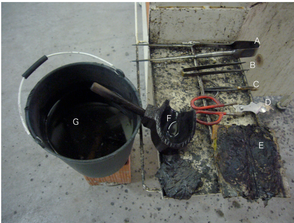
Figure 8. (A) Jacks, (B) Tweezers, (C) Bonsai Shears, (D) Diamond Shears, (E) Wet Newspaper, (F) Wood Blocks, (G) Water in bucket.
