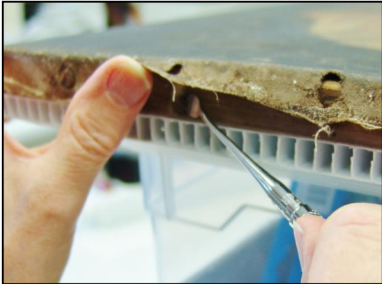
Fig. V.7. Normal light photographic detail of tack removal with metal spatula.
