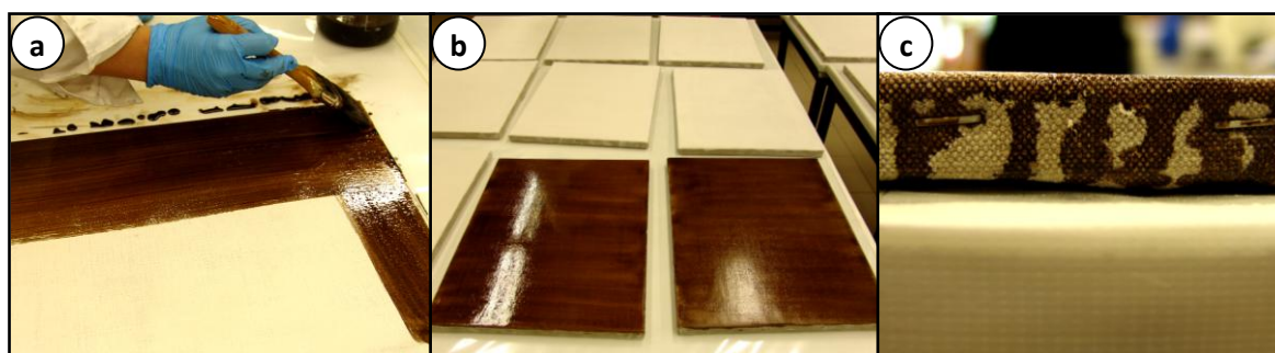
Fig. VII.5. a) Applying coloured varnish with brush; b) detail of 1 st application of varnish drying on model paintings; c) detail of varnish dripping.
