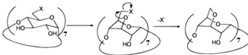
Figure 1.5: Conversion of a 6-substituted CD to a 3,6-anhydro CD. X is a good leaving group. [14]
