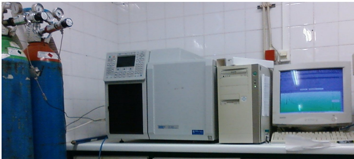
Figure 2.3 – Chromatograph CP-3800 used in GC analysis.
