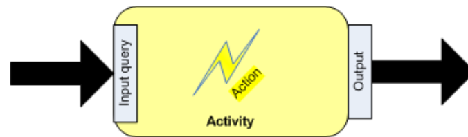
Figure 5.4: A detailed view of an activity. It may require an input or produce an output. In between, a certain action is executed.
