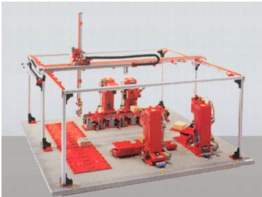
Figure 6.21: The MOFA France kit, deployed in its default configuration for simulation purposes. This kit provides several test components, like conveyor belts, cranes, machine tools, buffers or machine tables.
