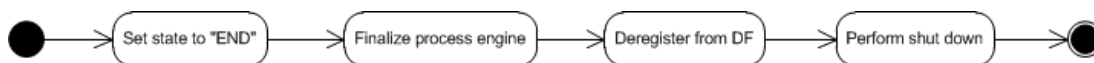
Figure 6.8: The finalization of the Process Agent. The steps shown in this UML state diagram are executed whenever the Process Agent performs a clean shut down.
