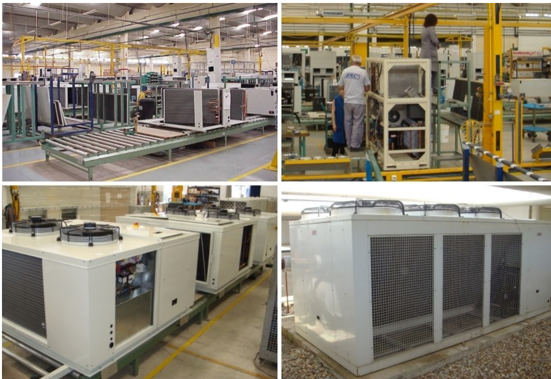
FIGURE 5.8. ASSEMBLING OF LARGE-SCALE AIR CONDITIONING UNITS.
