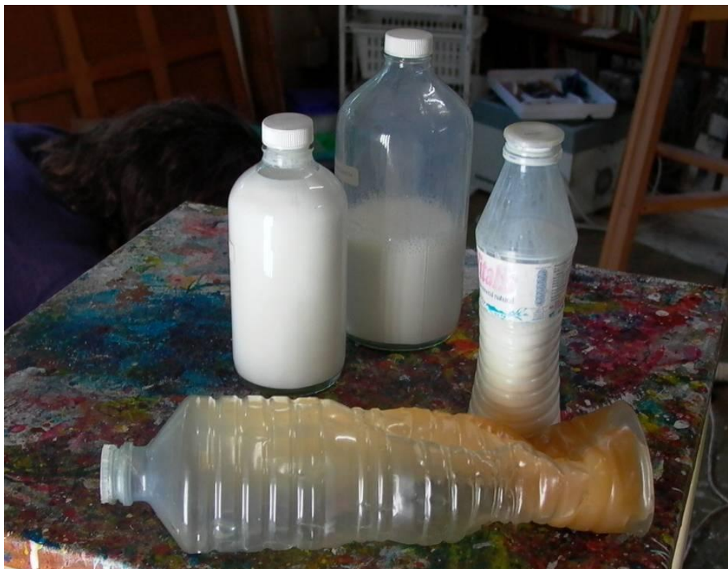
Figure 4.37. Examples of the vinyl emulsions supplied by Joaquim Simões stored in glass containers and vinyl emulsions supplied by Soberana kept in plastic bottles; in the smaller plastic bottle the emulsion had been diluted with extra water, the emulsion in the larger bottle has become a yellowish gel.
