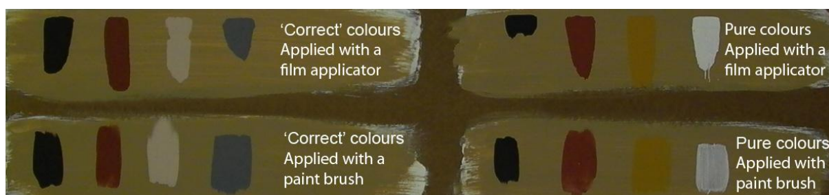
Figure 4.23 Colour reproductions, from the painting Os quintais , 1969, for which colour measurements were performed. The pure and 'corrected' colours were applied, both with paint brush and film applicator, on hardboard over a white preparation layer and background, reproducing Rodrigo's technique.
