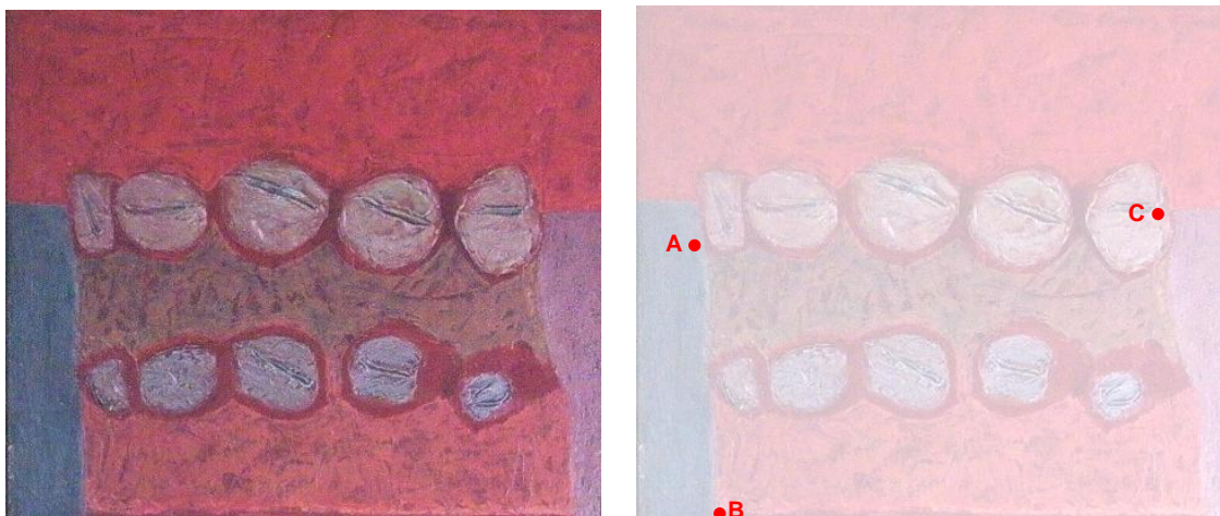
Figure VI.18. Untitled , 1961/62. Poly(vinyl acetate) on hardboard. Author's collection. \mu -sampling: A – green sample; B – red sample; C – whitish sample.
