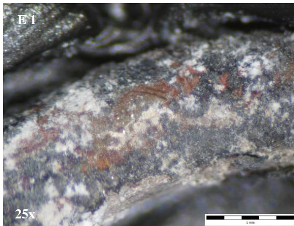
Figure 4.11 – Earring with dark grey and red corrosion products on the metallic surface (silver chlorides and cuprite), 25x.
