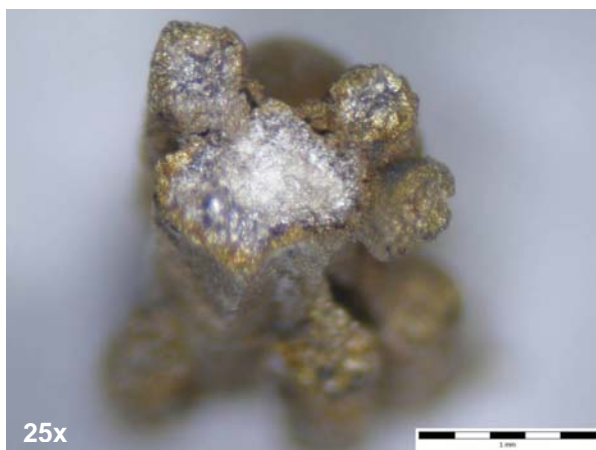
Figure 4.34 – Cross section of the F6' fragment n° 2, where is possible to observe the yellow patina only around the metallic surface.
