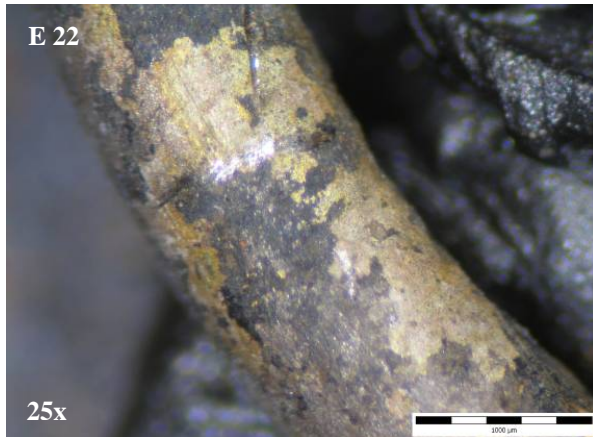
Figure 4.15 – Earring with yellow and dark grey patina, respectively, tarnishing and silver chlorides, 25x.
