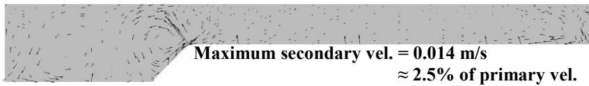
Figure 8. Secondary flow vectors obtained numerically in cross-section x = 7 m with EARSM turbulence model.
