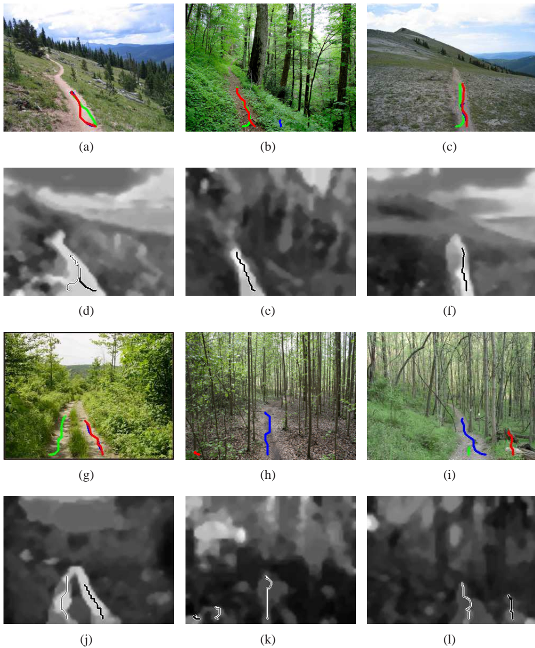
Figure 3.1: Input images (above) and respective saliency maps (below), where saliency is represented in grey level. These maps are the superposition of two conspicuity maps, one for colour and another for intensity channels. Each of these maps is searched for trails by agents (see Section 3.2), whose paths are described by the overlaid lines. Thicker lines refer to the most probable trail candidate, which appears in the input image in red. The best agent found on the intensity and colour conspicuity maps is represented in blue and green, respectively.
