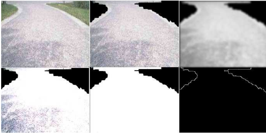
Figure 2.3: Border extraction process, as proposed in [Bartel et al., 2007]. Processing steps, from left to right, top to bottom, are: original image, green to black, gaussian blur, contrast enhancement, thresholding and border extraction
