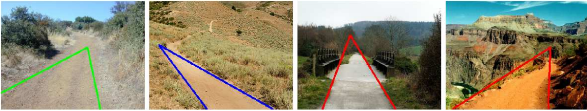
Figure 2.7: Appearance contrast method for trail detection as proposed in [Rasmussen et al., 2009]. The outputs of the detector are depicted as coloured triangles overlaid in the input image.
