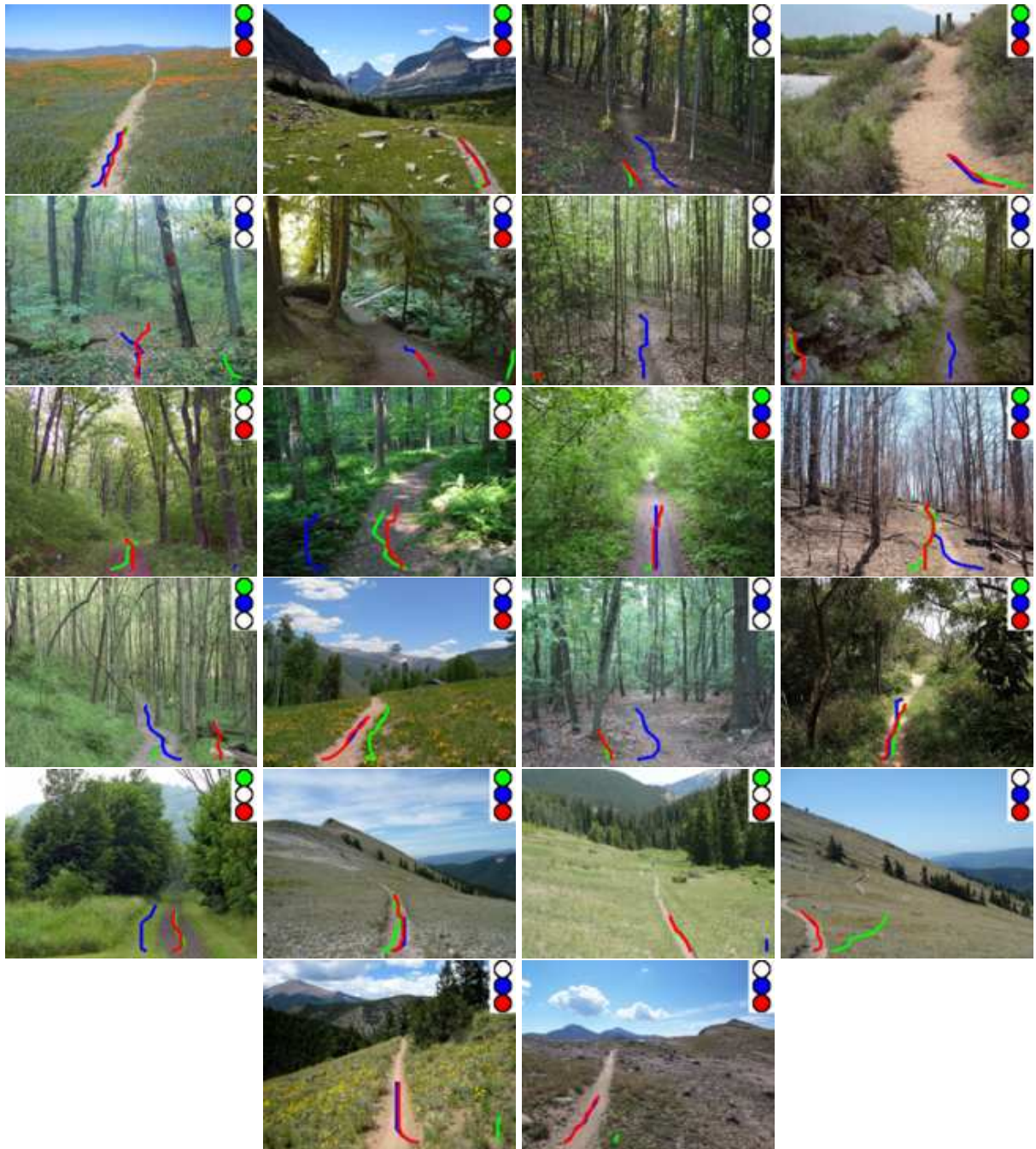
Figure A.8: Trail detection results (#29 to #50). The best agent's path in each map is superposed on the corresponding input image. Path colour is green, blue and red for the colour, intensity and saliency maps, respectively. In the top-right corner of each image, the presence of a filled circle with a given maps' colour, indicates that the best agent's path of the corresponding map correctly represents the trail.
