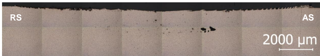
(C) D118-H: Pin completely overlaps SiC packed groove. Average particle size: 118.8 μm. Material: AA 5083-H111.
