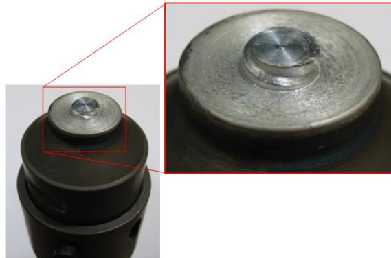
Figure 3.6 - Tool geometry used featuring a concave shoulder and a threaded cylindrical pin.
