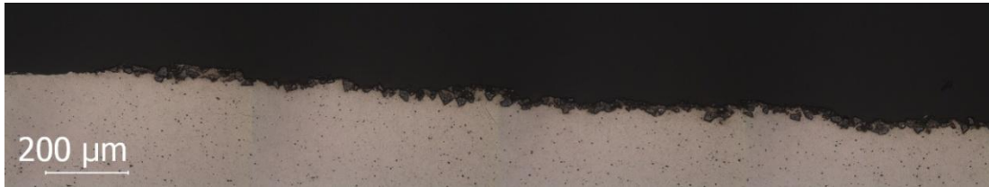
(B) D37-H: Pin completely overlaps SiC packed groove. Average particle size: 37.4 \mu\text{m} . Material: AA 5083-H111.
