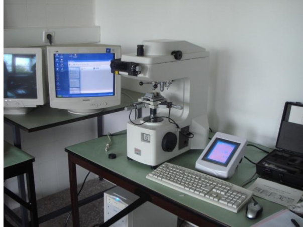
Figure 3.17 - Mitutoyo HM-112 Vickers micro-hardness testing machine.
