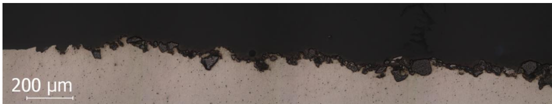
(F) D118-O: Pin completely overlaps SiC packed groove. Average particle size: 118.8 \mu\text{m} . Material: AA 5083 partially annealed at 400°C for 3.5h.
