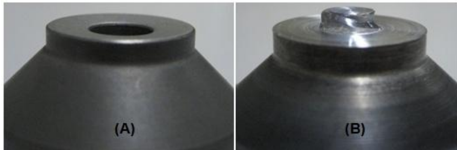
Figure 4.29 - Shoulder wear. As received from manufacture (A) and after trials (B).
