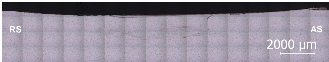
(A) D12-H: Pin completely overlaps SiC packed groove. Average particle size: 12.3 μm. Material: AA 5083-H111.
