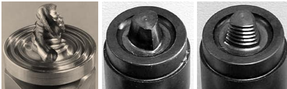
Figure 2.12 - Tool geometries patented by TWI [41-42].
