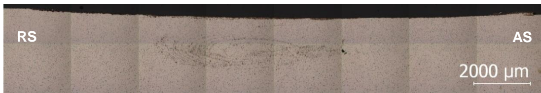
(E) D37-O: Pin completely overlaps SiC packed groove. Average particle size: 37.4 μm. Material: AA 5083 partially annealed at 400°C for 3.5h.
