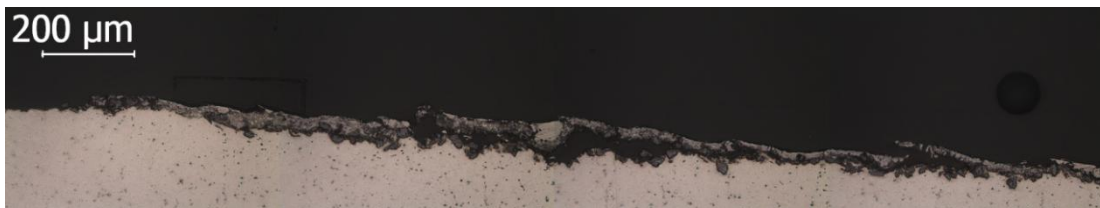
(E) D37-O: Pin completely overlaps SiC packed groove. Average particle size: 37.4 \mu\text{m} . Material: AA 5083 partially annealed at 400°C for 3.5h.
