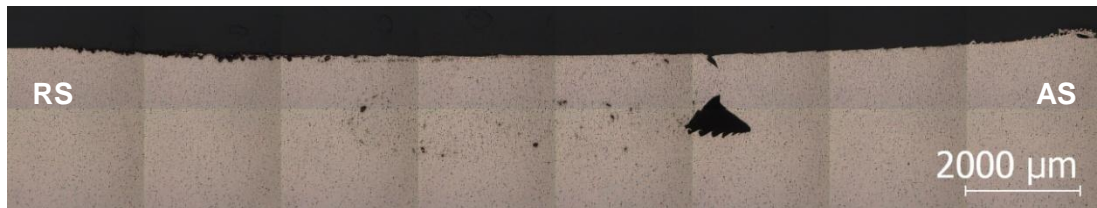
(F) D118-O: Pin completely overlaps SiC packed groove. Average particle size: 118.8 μm. Material: AA 5083 partially annealed at 400°C for 3.5h.
