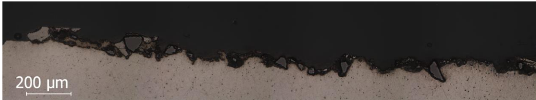
(C) D118-H: Pin completely overlaps SiC packed groove. Average particle size: 118.8 \mu\text{m} . Material: AA 5083-H111.
