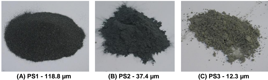
Figure 3.1 – Macroscopic appearance of silicon carbide particles used. 118.8 (A), 37.4 (B) and 12.3 μm (C) median sized.
