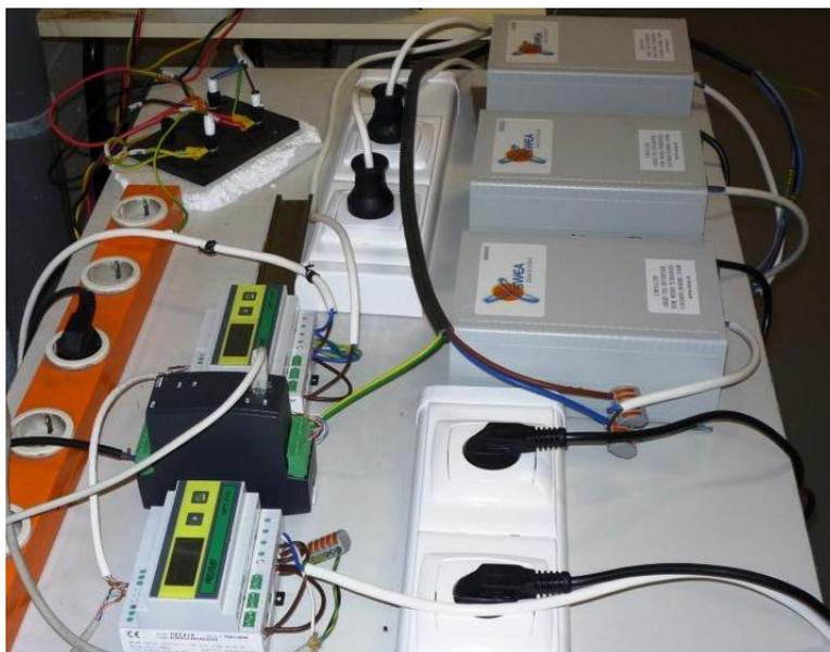
4.9: MONTAGEM DOS INVERSORES UWT-I-250 NO LABORATÓRIO DE ALTA TENSÃO DO DEE/FCT.
