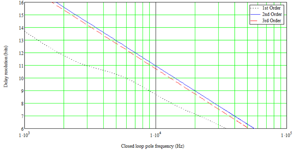
FIGURE 3.3: System resolution (in bits) of the DLL for different closed loop frequencies and a \Sigma\Delta modulator order of 1, 2 and 3.
