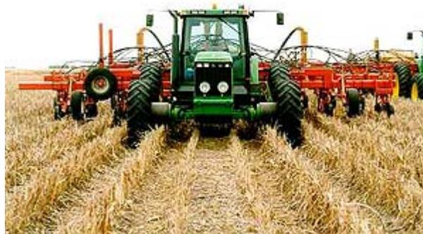
Figura 13 – Tractor com sistema CTF (*controlled traffic farming*) (DPI&F, 2004)
