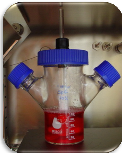
Figure 2.1 – Spinner flasks used for HEK293 culture, from Bellco®
