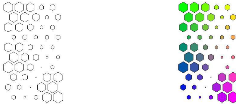
Figure 5 – Combining the distances matrix with similarities on the output space The size of each SOM unit on the U-matrix is function of the distances between that unit and its neighbours. Units that are near their neighbours (according to distances in the input data space) are greater than those who are far. This approach can be also combined with the use of colours.
