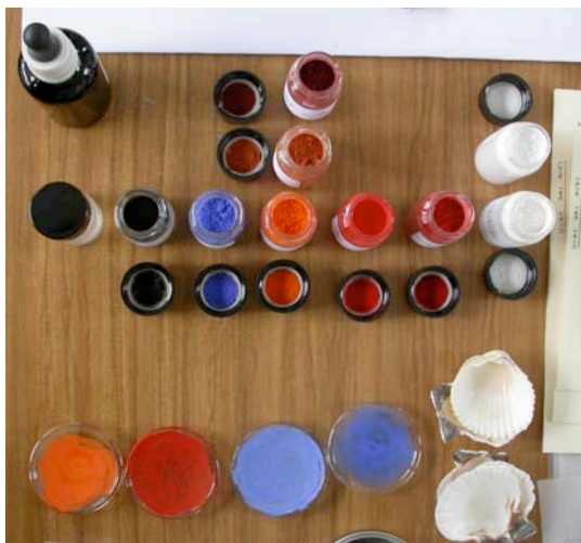
Figure 2.14. Some examples of paints made with minium , vermillion, lapis lazuli and white lead in different proportions, using parchment glue as a binder.
