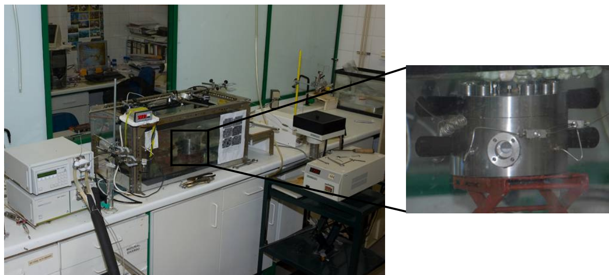
Figure 2.2 – Photograph of the experimental high pressure apparatus and detail of the high pressure cell.
