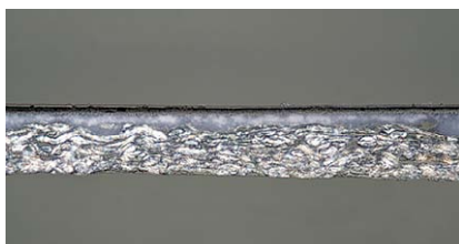
Figures 61 and 62 – Carbon and Carbro. Cross-sections in a 200x view, with BF reflected lighting (left to right). Both prints have a baryta coating to separate the gelatin layer from the paper support. In the Carbro example, the color layers are tightly overlapped.
