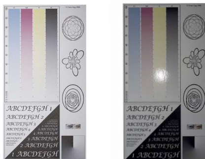
Figures 93 and 94 – Inkjet prints. Pigment based ink on a porous support and dye based ink on a swellable support (left to right). Normal view at 0° lighting. The irregular surface of the porous support doesn't reflect much light, but the opposite happens with the swellable support, that has a smooth surface.
