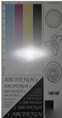
Figure 87 – D2T2 print. Normal view at 0° lighting. Because it is an RC coated sample, the surface is smooth and can reflect light easily.
