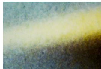
Figures 160-161 – Agfacolor, Cibachrome (left to right). 50x view at 90° lighting. Using a plastic coating over a paper base core prevents the print's surface from showing irregularities related to those fibers.
