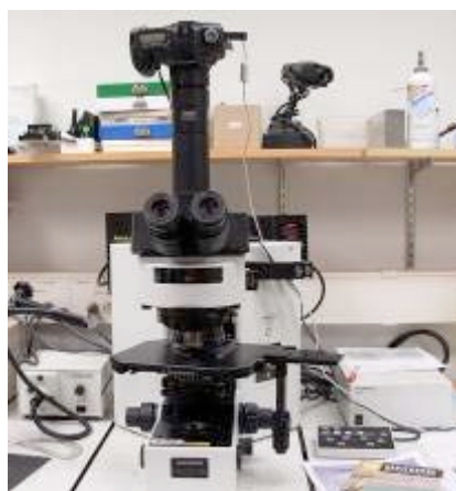
Figure 119 – Olympus AX70 compound microscope with digital camera attachment.
