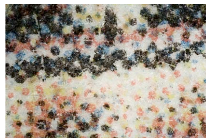
Figure 30 – Color offset lithograph. 50x view at 45° lighting. The pattern isn't as sharp as the one shown by letterpress halftone prints.
