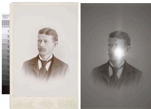
Figures 42 and 43 – Collodion POP print. Normal view at 45° and 0° lighting (left to right). This print has a pink tinted baryta layer. Because it is has a very smooth surface, it shows high gloss under 0° lighting.
