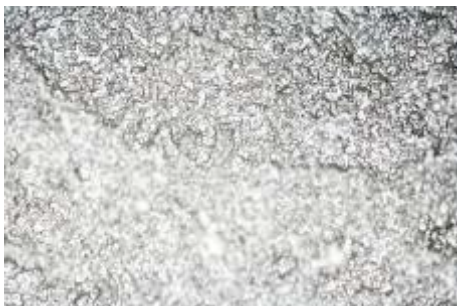
Figures 122 and 123 – B&W silver gelatin print from a 1937 Kodak Sample Book, named Kodak Royal Bromide Grade T. Left: regular image, with out of focus bottom left corner; Right: composite image, all focused. Non polarized BF, at 200x. Not on www.digitalsamplebook.com .
