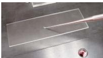
Figure 128 – Collecting sample with dental pick.
