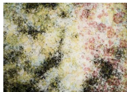
Figure 19 – Color collotype. 50x view at 45° lighting. Each color layer presents the reticulation pattern.
