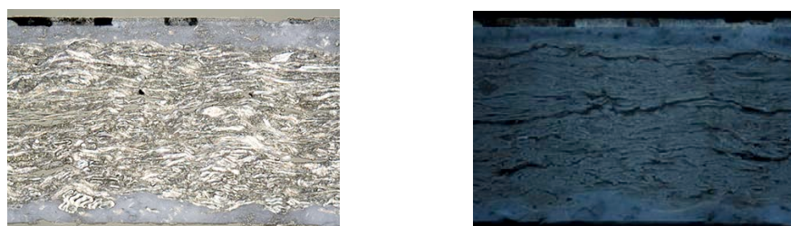
Figures 34 and 35 – Letterpress halftone. Cross-sections at a 200x view, in BF reflected light and DF-UV light (left to right). The paper used for this print had an extra coating to prevent the ink from penetrating into the paper fibers. It is not, however, a fluorescent material.
