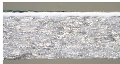
Figures 61 and 62 – Carbon and Carbro. Cross-sections in a 200x view, with BF reflected lighting (left to right). Both prints have a baryta coating to separate the gelatin layer from the paper support. In the Carbro example, the color layers are tightly overlapped.
