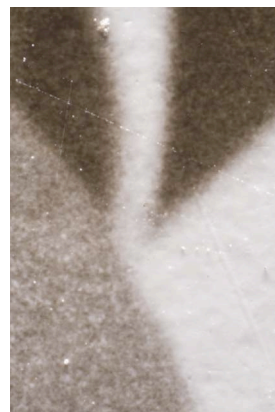
Figure 44 – Collodion print at 90° lighting , 50x. No paper fibers are shown due to the baryta layer.
