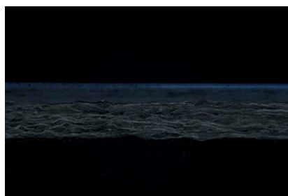
Figure 124 – Gelatin P.O.P. print under UV lighting. DF Reflected light at 200x. The top gelatin layer shows some fluorescence, while the remaining layers of the print (baryta layer and the paper support) don't show the same phenomenon.
