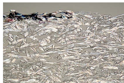
Figure 92 – Iris print. Cross-section at 200x, with BF reflected light. The ink is absorbed by the top fibers. Also, this paper support is relatively thick.
