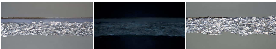
Figures 45 and 46 – Collodion POP print. Cross section in a 200x view at BF reflected lighting and DF-UV lighting (left to right). This print has a relatively thick baryta layer to cover the support. Under UV light, it doesn't fluoresce.
