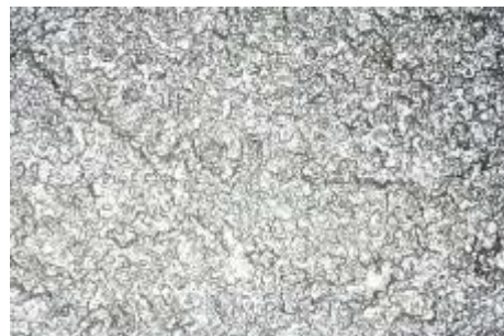
Figures 122 and 123 – B&W silver gelatin print from a 1937 Kodak Sample Book, named Kodak Royal Bromide Grade T. Left: regular image, with out of focus bottom left corner; Right: composite image, all focused. Non polarized BF, at 200x. Not on www.digitalsamplebook.com .
