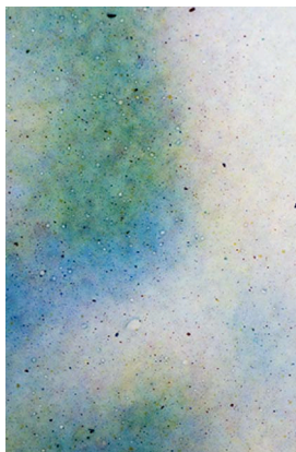
Figures 59 and 60 – Carbro. 50x view at 45° and 0° lighting (left to right). At 45° it is possible to observe pigment particles and missregistration between the blue and yellow layers. At 0° the image shows differential gloss.
