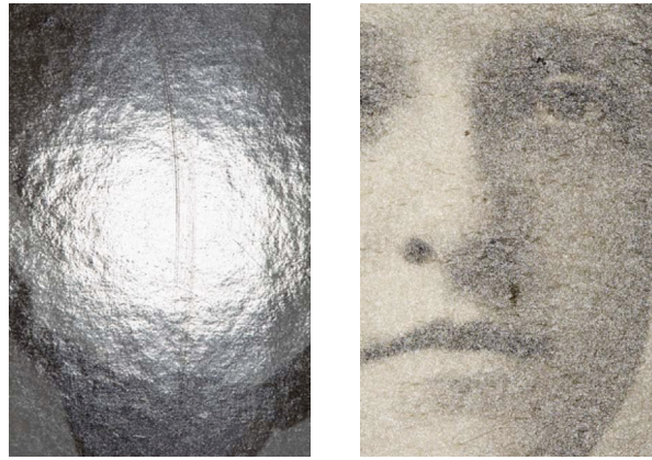
Figures 111 and 112 – Collodion P.O.P. and matte collodion prints (left to right) at the macro shot, at 0° lighting. Because the surface is so smooth on the collodion P.O.P. sample, light is reflected almost entirely, and the silver image is barely seen. The opposite happens with the matte collodion print.
