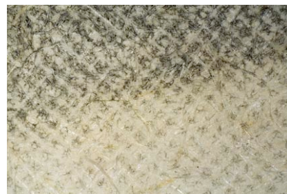
Figure 26 – Rotogravure. 50x view at 45° lighting. The image is formed by squares with ink, separated by perpendicular lines with no ink.
