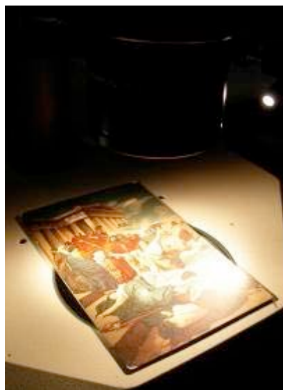
Figure 131 – Print observation under the stereomicroscope. In this case, the fiber optics are positioned in a close to 45°, to observe image structure of the print.
