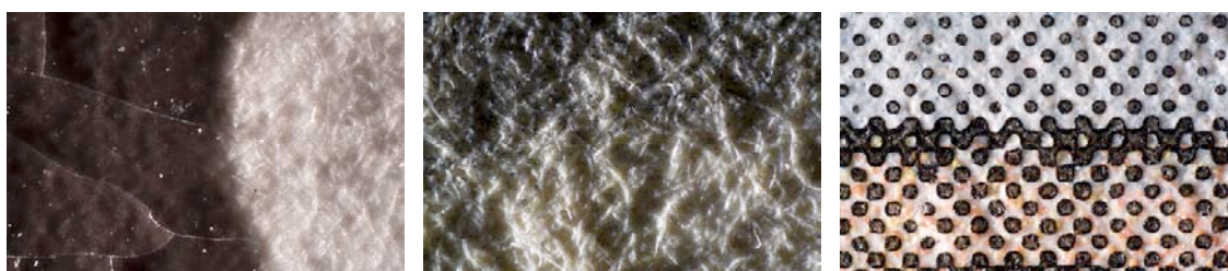
Figures 31-33 –Woodburytype, rotogravure and letterpress halftone prints (left to right). 50x view at 90° lighting. Fibers are visible on the non image areas of the Woodburytype, all across the rotogravure surface, and hidden in the letterpress halftone print, due to an extra coating.
