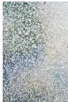
Figures 59 and 60 – Carbro. 50x view at 45° and 0° lighting (left to right). At 45° it is possible to observe pigment particles and missregistration between the blue and yellow layers. At 0° the image shows differential gloss.
