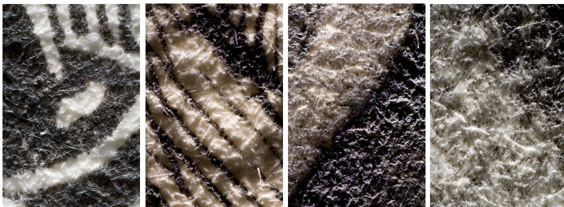
Figures 10-13 – Woodcut, engraving, etching and lithograph (left to right), seen at 50x with 90° lighting. In all the examples paper fibers are visible, even under the ink layer.
