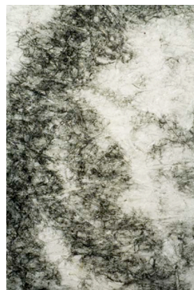
Figure 24 – Photogravure. 50x view at 45° lighting. The aquatint grain pattern is observed.
