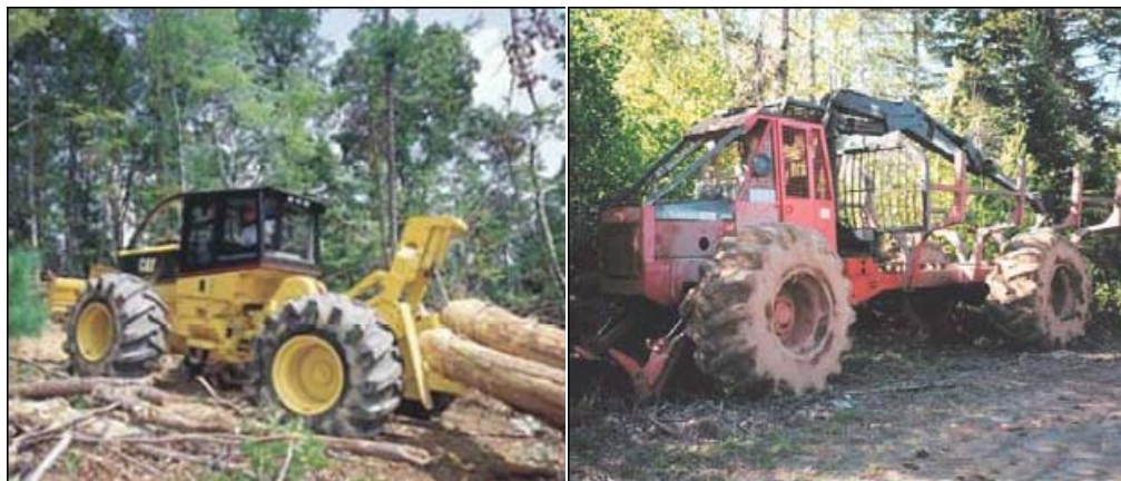
Figura 3.2 Skidder de cabo (esq.) e forwarder (dir.) (RE Consulting, 2007).
