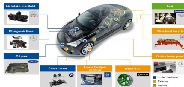
Figure 1.1. Light-weight components targeted by today automotive manufacturers [12]
