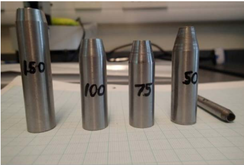
Figure 2.12. Picture of the bespoke extraction tools used to remove bryozoans from PVC panels to allow mass (AFDM) measurements to be made
