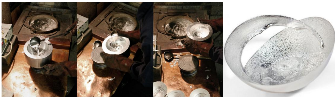
Figure 6-10: Slush cast bowl, process and finished bowl, by Ian McIntyre, 2008
