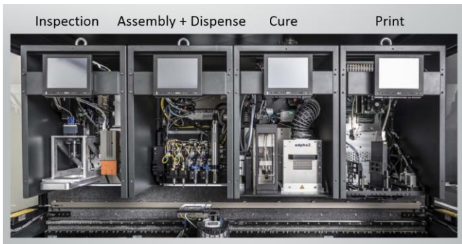
Figure 3: Interior view of the the NextFactory 3D manufacturing system showing modular nature of printing, cure, assembly, dispense and inspection
