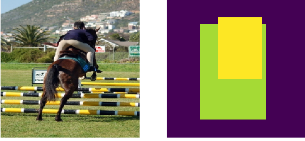
Figure 4. Example of weak segmentation ground-truth. Left: Input image with a size of 300 \times 300 , with a person and a horse. Right: Segmentation ground-truth for the left image, with a size of 38 \times 38 ; the pixels locate in both person and horse bounding-boxes will be assigned to person class since its bounding-box is smaller.
