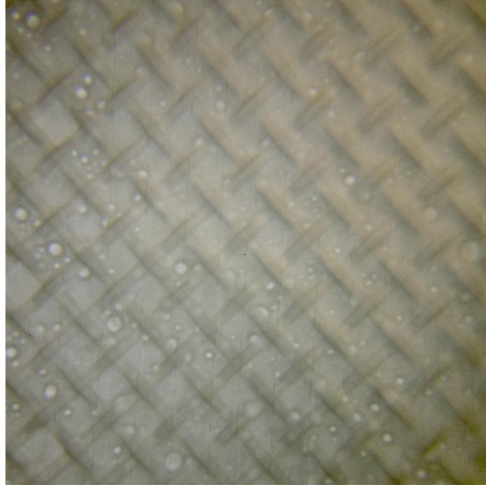
**Figure 10.** Hydrophobic surface picture with temperature conditions at  $T_H = 70^\circ\text{C}$ ,  $T_C = 20^\circ\text{C}$  showing the small droplets found on the surface.
