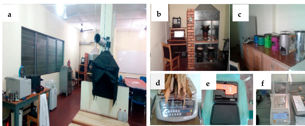
Figure 2. (a) Testing facility, including (b) test hood (LEMS), (c) improved cookstove library, (d) large-capacity scale, (e) Delmhorst J-2000 moisture meter, and (f) precision balance.
