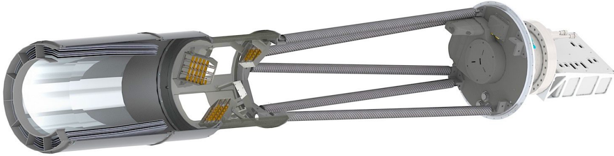
Figure 1. Cutaway rendering of the REDSoX Polarimeter from engineering design, showing the optics at left, gratings (in gold), the optical bench, the focal plane baffle (with three slits for dispersed events) over the pendulum valve for the detector chamber, and the back of the detector chamber with the electronics box. The top and bottom grating groups intercept opposite 60^\circ sectors of focused X-rays, dispersing them through the baffle slit to the left of the central (rectangular) aperture for 0th order. For clarity, only a few mirror shells and grating groups are rendered.
